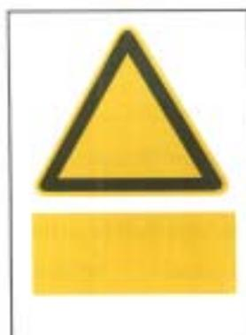
FIG. 11 LAYOUT FOR A COMBINATION SIGN WITH THE SUPPLEMENTARY SIGN BELOW THE SAFETY SIGN
