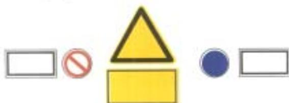
FIG. 10 POSITION ASSIGNMENT OF A SUPPLEMENTARY SIGN
