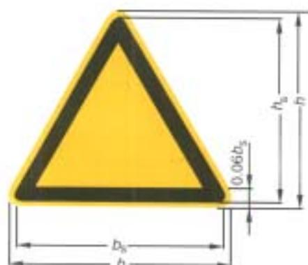
FIG. 3 LAYOUT REQUIREMENTS FOR A WARNING ACTION SIGN
