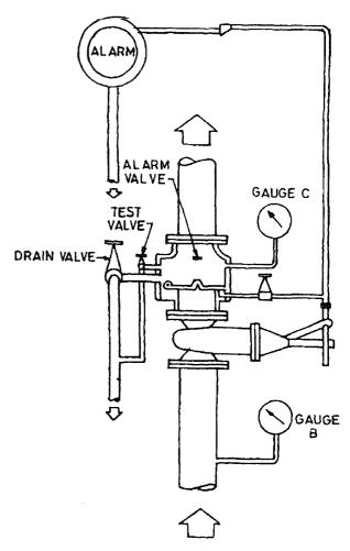
Fig. 29 Sprinkler Installation Valve Assembly
