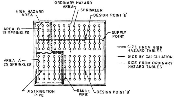
FIG. 12 PRECALCULATED HIGH RISE INSTALLATION (AMAO FED BY TWO DISTRIBUTION PIPES)
