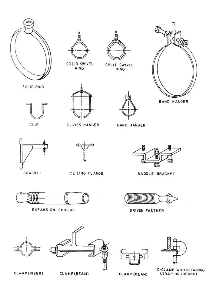
FIG. 15 COMMON TYPES OF PIPE HANGER EQUIPMENT
