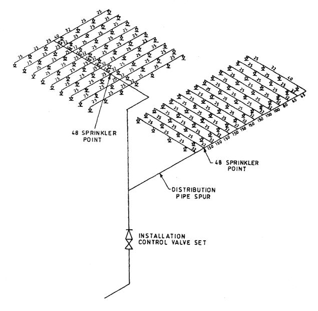
Fig. 23 Design Points in High Hazard Installation with Pipework Sized from Tables 32 and 34
