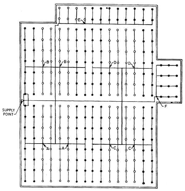
FIG. 21 DESIGN POINTS IN AN OH INSTALLATION
