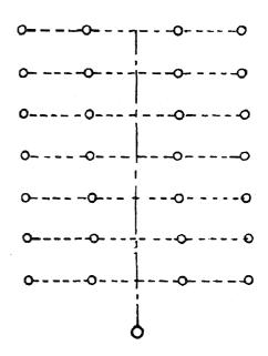
FIG. 4 TWO END-CENTRE WITH END FEED
